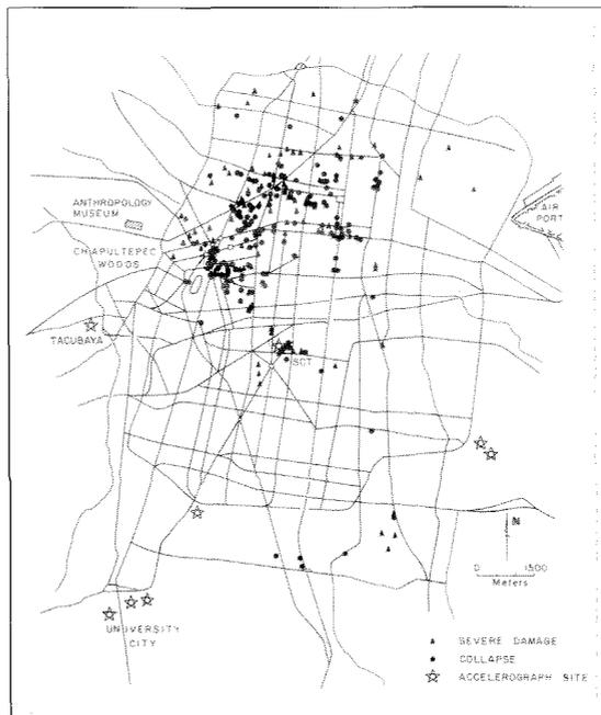
Figure 2 (left): Distribution of severe structural damage and sites where records of the strong ground shaking were obtained. Only some of the major streets of Mexico City are drawn. Damage is confined to areas on the old lake bed.
