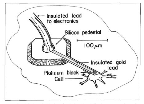
**P**ine and Rutledge hope that the diving board electrode will allow long-term recording and stimulation of a neuron maintained in cell culture.
