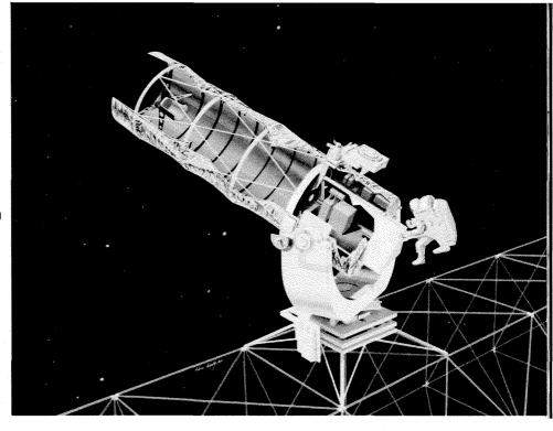
By the mid-1990s the Circumstellar Imaging Telescope, with its 1.9-meter supersmooth mirror, could orbit the Earth as an attached payload on the Space Station.
