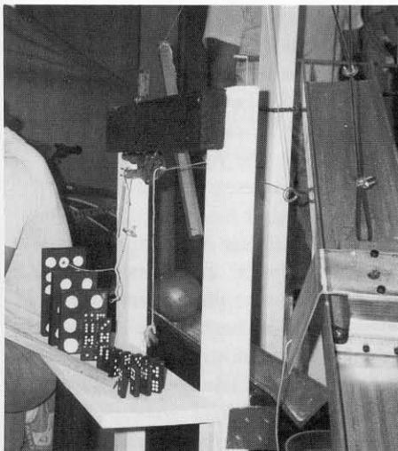
**. . . a line of increasingly larger dominoes, the last of which opens the jaws of the vice-grips, releasing the string which lowers the boom on the shotput, sending it along the channel. . .**
