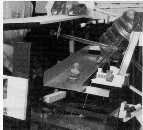
**. . . 5-gallon water bottle, filling the aquarium until the toilet-tank float pulls a string to lift a hinge sending a toy off-road vehicle plunging down the hill into a golf ball, which rolls down a ramp to tip over the first of. . .**
