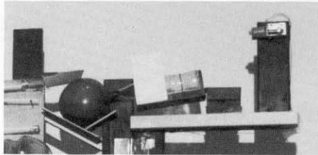
**. . . closing a circuit that makes a pinball plunger knock over a soda bottle. Vinegar in the bottle mixes with baking soda in the balloon taped to the bottle neck. The inflated balloon tips a steel ball bearing out of the manila envelope. . .**
