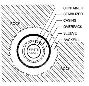
At Yucca Mountain (left) in Nevada. groundwater must flow 50 km before coming to the surface, which would take 100,000 years. Unseparated nuclear waste could be buried (right) at such a site in borosilicate glass surrounded by a container built to last several centuries. Then comes stabilizer, overpack, and a claylike backfill estimated to last 100,000 years.
