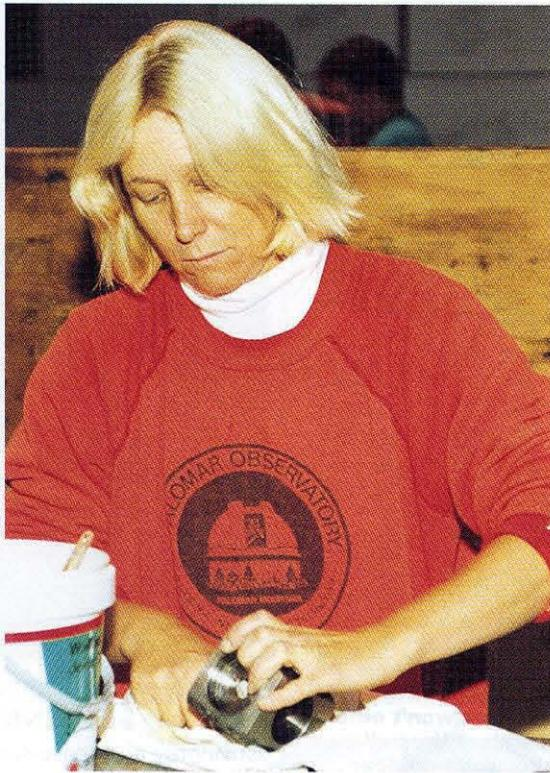
**Top: Facilities maintenance mechanic Dana Cunev gets the old grease off with paint thinner. Eventually, rags and paintbrushes give way to a wire toothbrush to clean out all the holes and cutouts. Some of the parts have a lot of holes and cutouts. Middle: Weber uses the arbor press to seat a bearing. Bottom: Petrie and Weber dismantle a central gimbal assembly, a process not unlike opening a Chinese puzzle box.**
