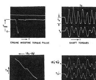
STRESS-STRAIN CURVE FOR SHAFT NO. 3
