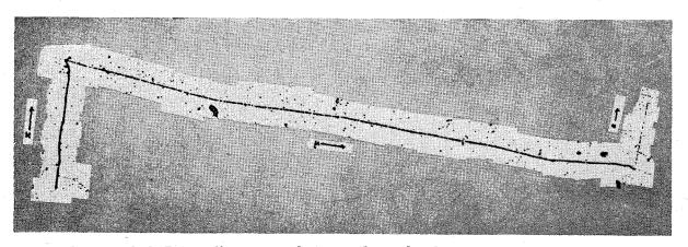
In Bristol, England, C. F. Powell is now analyzing tracks produced by mesotrons in emulsions of photographic plates. The track above shows how the decay of a pi mesotron (left) produces a mu mesotron (long horizontal line), which decays in turn to produce the electron whose track is shown at the right.
