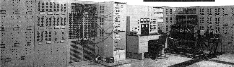
This is one of two control panels for the Electric Analog Computer located in Caltech's Analysis Laboratory.
