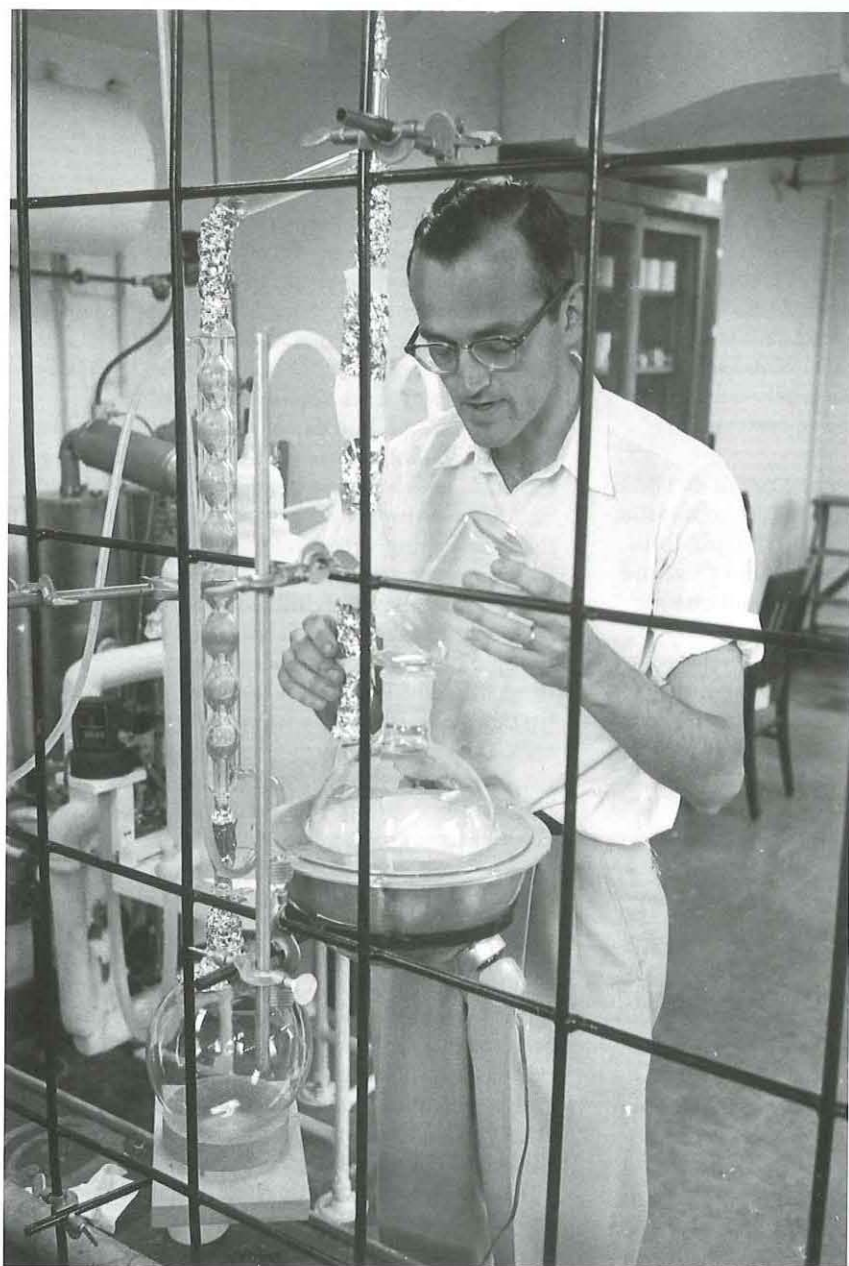
Patterson uses a distillation apparatus to purify reagents in his Caltech lab in 1957. He didn't trust the purity of commercial chemicals, so he redistilled them.
