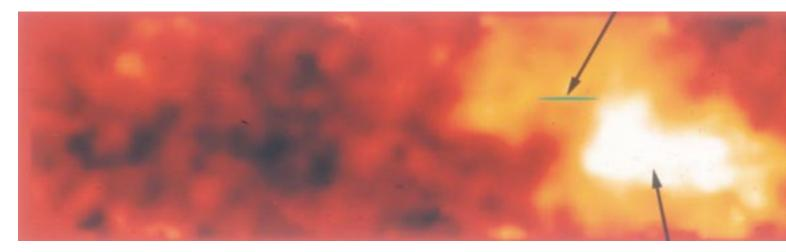
Far right: The Stardust mission will visit comet Wild 2 in 2004 and return to Farth with hits of comet dust captured in the apparatus projecting above the conical return capsule. Embedded in that holder, shown at lower right, is an airy silica substance called aerogel. When the particles encounter the aerogel at 14,000 miles per hour (right), they slow down and are trapped.
