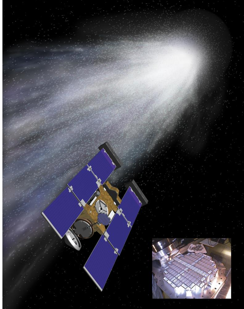
Comet Wild 2 will be safely past its active peak and on its way back into the deep-space deep freeze when Stardust catches up with it. The spacecraft will fly through the comet's coma, or dust cloud, about 150 kilometers in front of the nucleus. The inset shows the collector being filled with aerogel.
