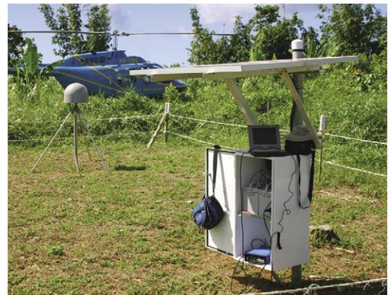
**A typical GPS installation. The gray dome on the tripod in the background houses the GPS unit proper, and the open cabinet under the solar panel contains the electronics.**
