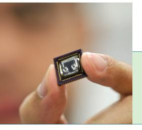
An up-close representation of the optofluidic microscope. The green specimen flows across the gray metal sheet. The detector underneath captures images of the specimen through the holes.
