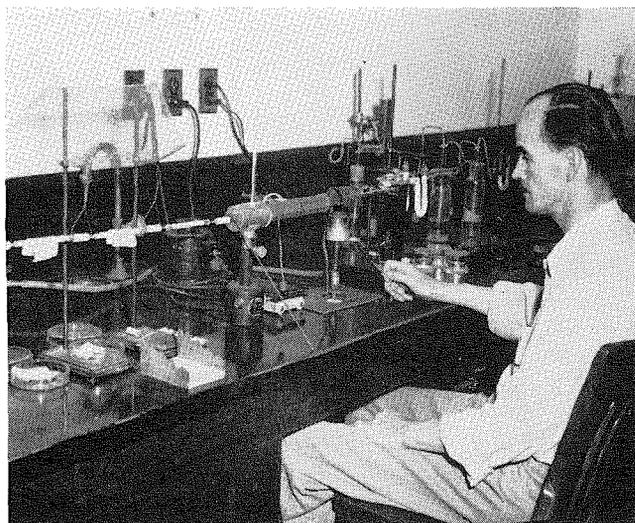
Since the most numerous compounds found in biological material are compounds containing carbon and hydrogen, the combustion analysis of carbon and hydrogen is highly important to the organic chemist and biologist. Assistant Swinehart is carrying out such a combustion analysis.
