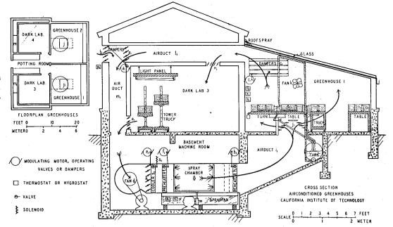
Floor plan of the present greenhouses (left side faces north) and cross median section through house "1" and room "3".
