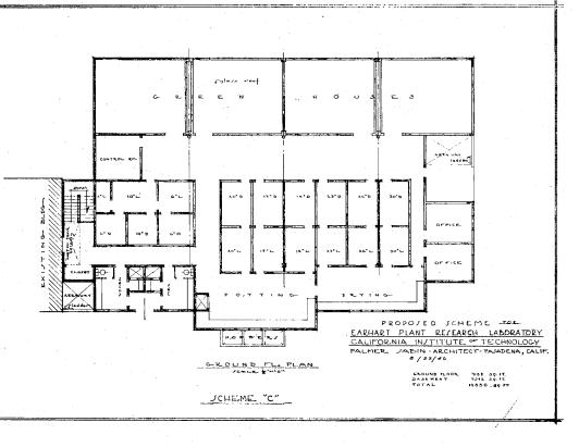
Floor plan of the projected Earhart Plant Research Laboratories at the Institute. Illustrated is the arrangement around a central hallway of four separate greenhouses and 18 light and dark rooms for controlled temperatures ranging from 2° to 30°C.
