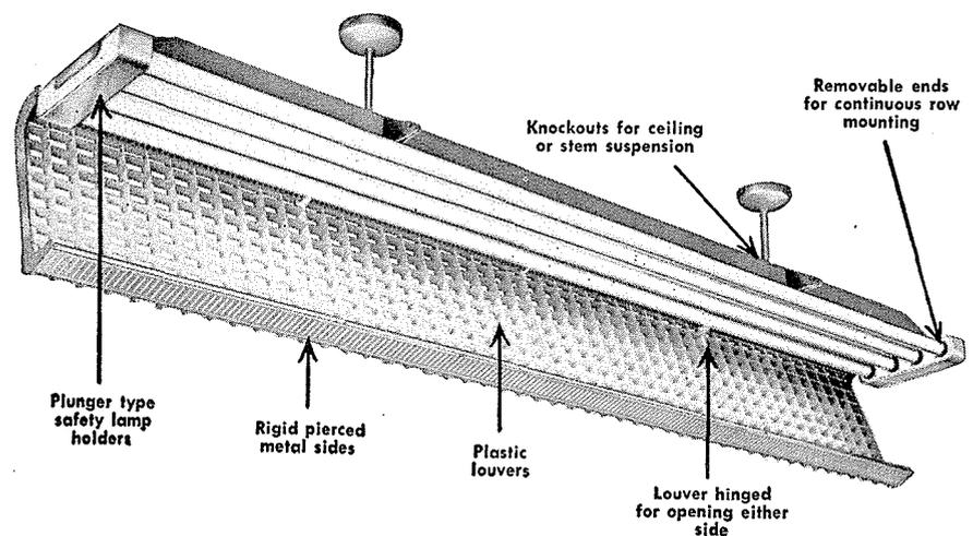
This outstanding luminaire utilizes the brand new high output 75 watt, 425 m. a. T-12-96" fluorescent lamp. It is scientifically engineered to produce the utmost in lighting quality and efficiency.
