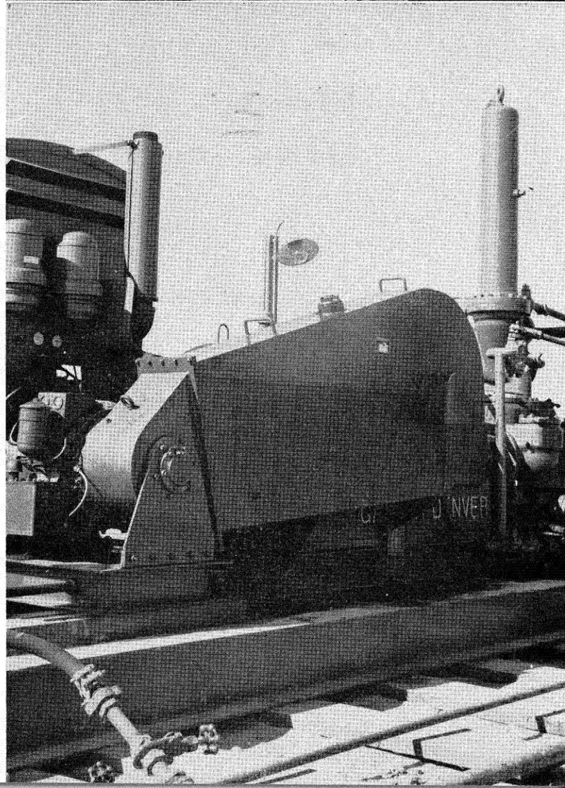
strain is greatest at stalled speeds, but is substantial up to a speed equal to the reverse speed of the craft. The hydraulic torque converter insures maximum pull on the anchor line at all times and also sufficient speed on the spooling drum to make sure that all slack is taken up as the boat is floated by the combination of the anchor line pull and action of the waves.
