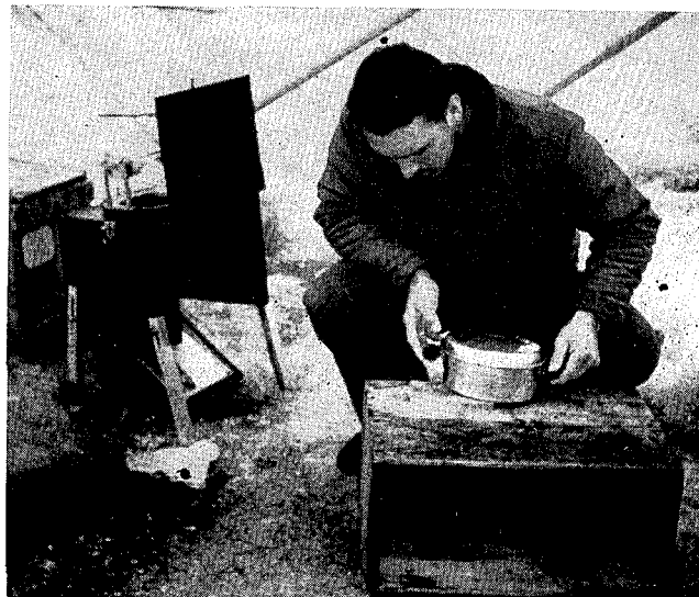
Preparing a thin-section of ice for study on an oversized universal stage, which is shown at the left.
