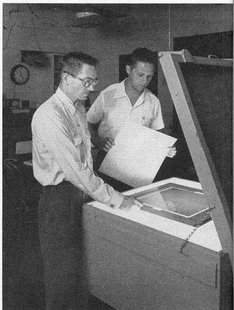
James McClanahan and his assistant, Hendrik Rubingh, using a vacuum printer to process Survey photographs.
