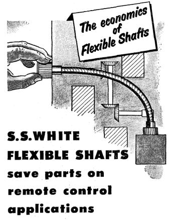
Just compare the simplicity of the flexible shaft control, shown above, with the combination of rods, bevel gears, pulleys and belts that might otherwise be necessary. The savings in parts and costs are obvious. What's more the flexible shaft is less complicated, needs no alignment; is easier to install and gives more freedom in mounting the coupled parts where desired to assure better and more convenient operation.
