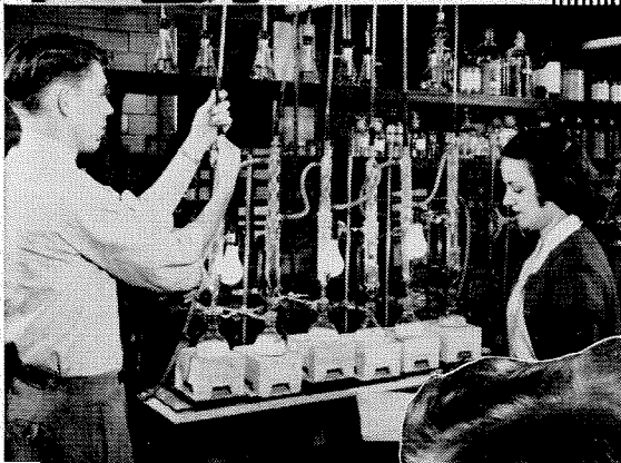
Testing action of Per-chloroethylene on various metals.
