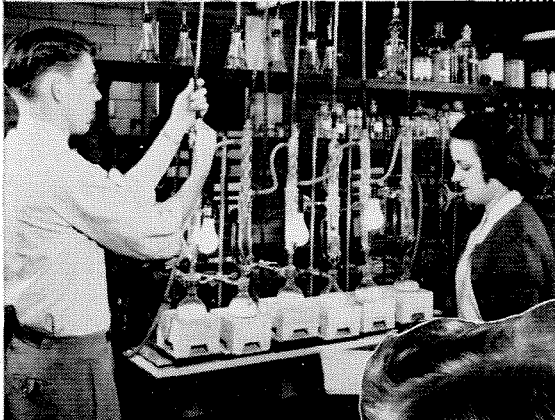
Testing action of Perchloroethylene on various metals.
