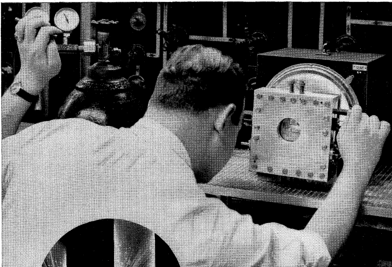
This Sperry engineer is applying the fundamentals of hydraulics to determine oil flow characteristics at high pressure. Here he introduces nitrogen to the hydraulic fluid in a complex valve to make flow patterns visible for study.
