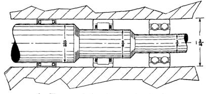
1. Illustrates the fact that for a given housing bore size, a larger and, therefore, stiffer shaft can be used with Needle Bearings than with a roller or ball bearing.
