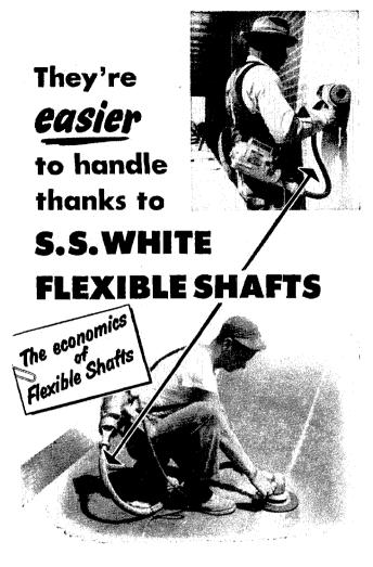
• LIGHT WEIGHT AND MOBILITY are essential features of any portable tool. That's one reason why the manufacturer of these concrete surfacers uses S.S.White flexible shafts to transmit power between the motor and the working head. As he puts it, the flexible shafts "provide flexibility of movement for the operator and eliminate the need for holding the motor unit which is the heaviest part of the equipment."
