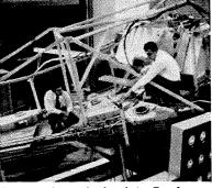
Flying fuel jig developed in Republic's laboratories to simulate actual conditions of in-flight refueling.
