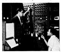
Analogue computer at Republic simulates flight conditions mathematically, materially shortens flight test period.
