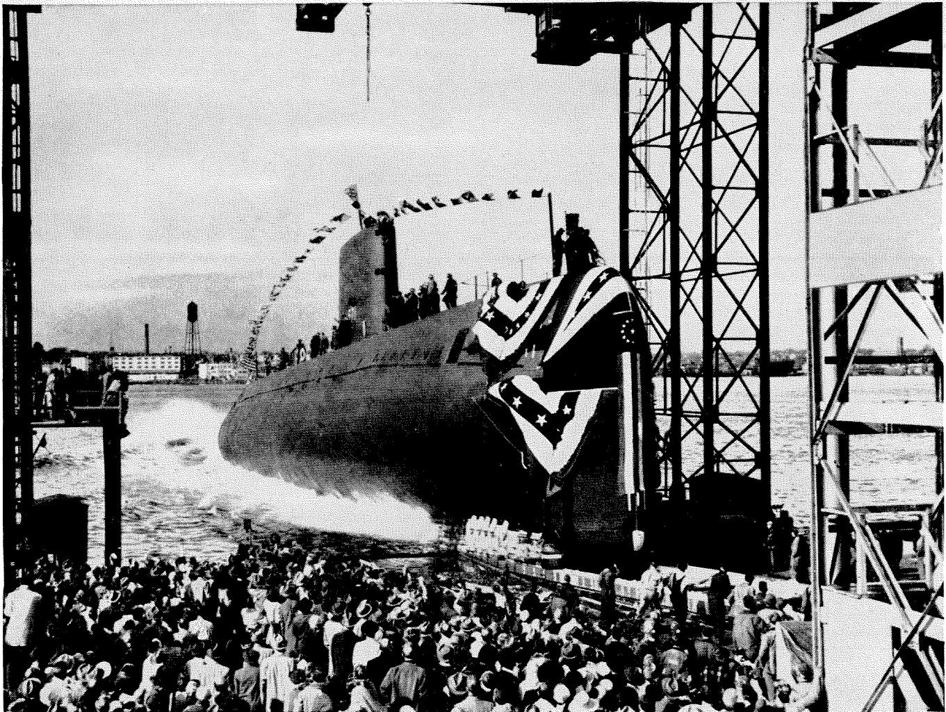
SLIDING DOWN THE WAYS at Groton, Conn., goes the USS Nautilus, newest and fastest member of our underseas fleet. During welding, Worthington heavy-duty turning rolls rotated the hull sections.
