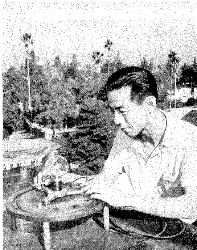
Dr. Eugene Loh checks the pyroheliometer on Caltech's solar furnace, which gives a continuous record of the intensity of solar radiation.
