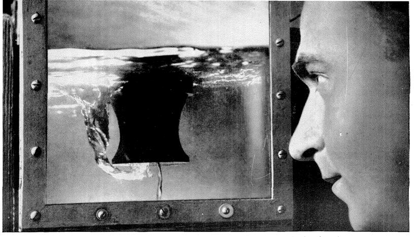
A WHIRLPOOL SPIRALS into the inlet of a model pump. This unique picture shows how air, a common cause of pumping trouble, was carried into the pump in ...
