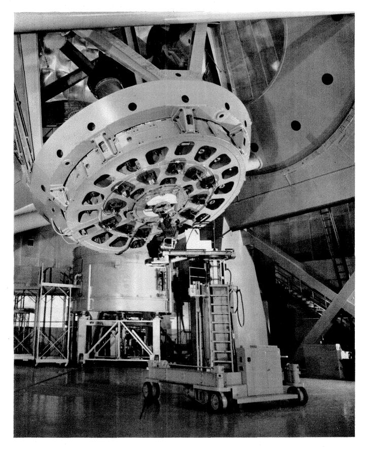
Besides the prime focus, there are several other types of observation stations. Here the astronomer is at the Cassegrain focus on the underside of the 200-inch mirror. In the chair designed especially for this station, the astronomer is preparing to take photographs.
