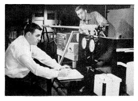
Mechanical Research Engineer W. M. Watkins (left) directs Research Mechanic Earl Rollo in operating Lockheed's new Hailstone Gun during a test on the effect of hailstones on new types of plastic radome "skin." The gun, which was designed by Watkins and Mechanisms Group Engineer G. W. Louthan, fires up to five hailstones spaced 25 feet apart at speeds ranging from 270 to 500 mph. The hailstones, which are made in the gun, can be varied in size from  $\frac{36'}{36'}$  in diameter.
