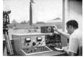
Electronics Research Engineer Irving Alne records radiation antenna pattern on Lockheed's Radar Range. Twenty-two foot plastic tower in background minimizes ground reflections, approximates free space. Pattern integrator, high gain amplifier, square root amplifier and logarithmic amplifier shown in picture are of Lockheed design.
