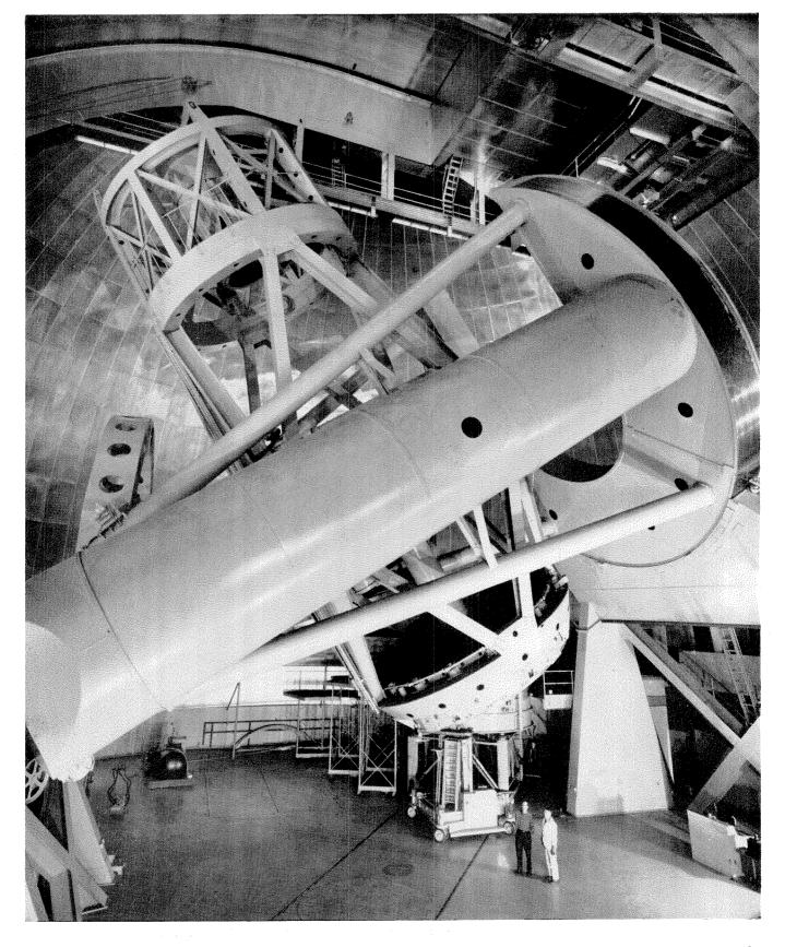
The 200-inch telescope sits for its latest portrait. At the top of the tube, above, is the prime focus cage, where the astronomer works. On the opposite page is the cage itself, where the astronomer is preparing to take a series of direct photographs. The 200-inch is the only telescope in the world in which an observer actually rides while working.
