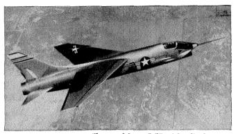
**CHANCE VOUGHT F8U** — Powered by a J-57 with afterburner, the Crusader is the Navy's fastest carrier-based fighter.
