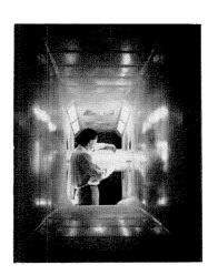
**C. H. Fish, design engineer** assigned to Lockheed's Icing Research Tunnel, measures impingement limits of ice on C-130 wing section. The tunnel has a temperature range of  $-40^{\circ}$ F. to  $+150^{\circ}$ F, and maximum speed of more than 270 mph. It is the only icing research tunnel in private industry.
