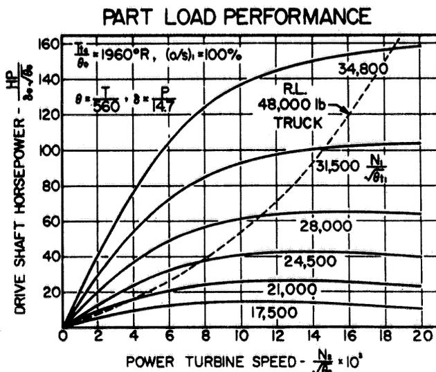
Output vs power turbine speed. R.L. = road load. Numbers on curves are compressor speeds (Ref. 12) (Ford)
