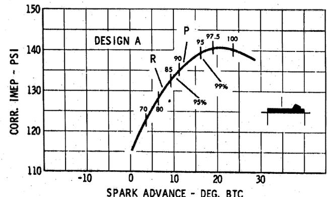
Comparison of flat (Design A) and compact (Design B) combustion chamber .9:1 compression ratio; 1,000 rpm. R = Regular, P = Premium (1954 level) 99 percent = 99 percent of maximum i.m.e.p. (indicated mean effective pressure) (Ref. 9)
