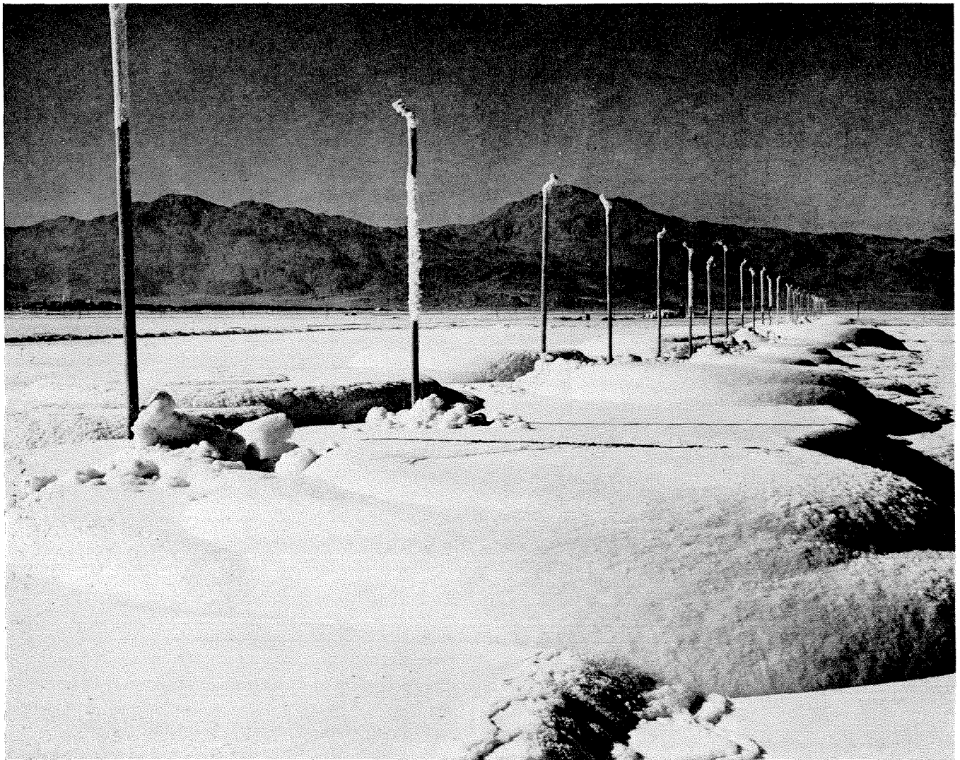
Glauber salt operations of the American Potash and Chemical Corporation at Searles Lake, California. In winter, when temperatures are sufficiently low, fossil brine is pumped from the crystalline salt body below and sprayed into the air, precipitating Glauber salt, which is "harvested" in spring or summer. In the plant in the background the fossil brine is processed for its yield of potassium salts, borax, sodium carbonate, lithium compounds and other valuable mineral materials.
