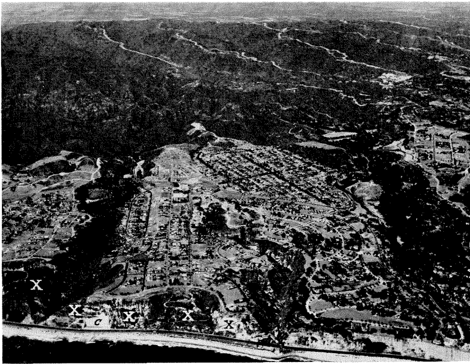
Settlement of coastal terraces in the Pacific Palisades area, 1946. Large landslide masses (X) face the ocean, and a steep-walled cut (C) exposes old slide debris.
