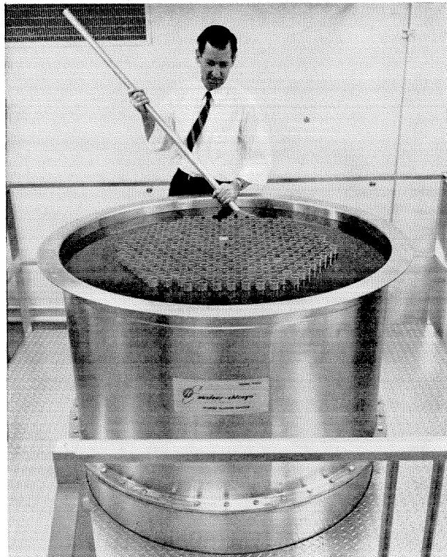
Harold Lurie, associate professor of applied mechanics, assembles a pattern of uranium-filled tubes in Caltech's new subcritical nuclear reactor.
