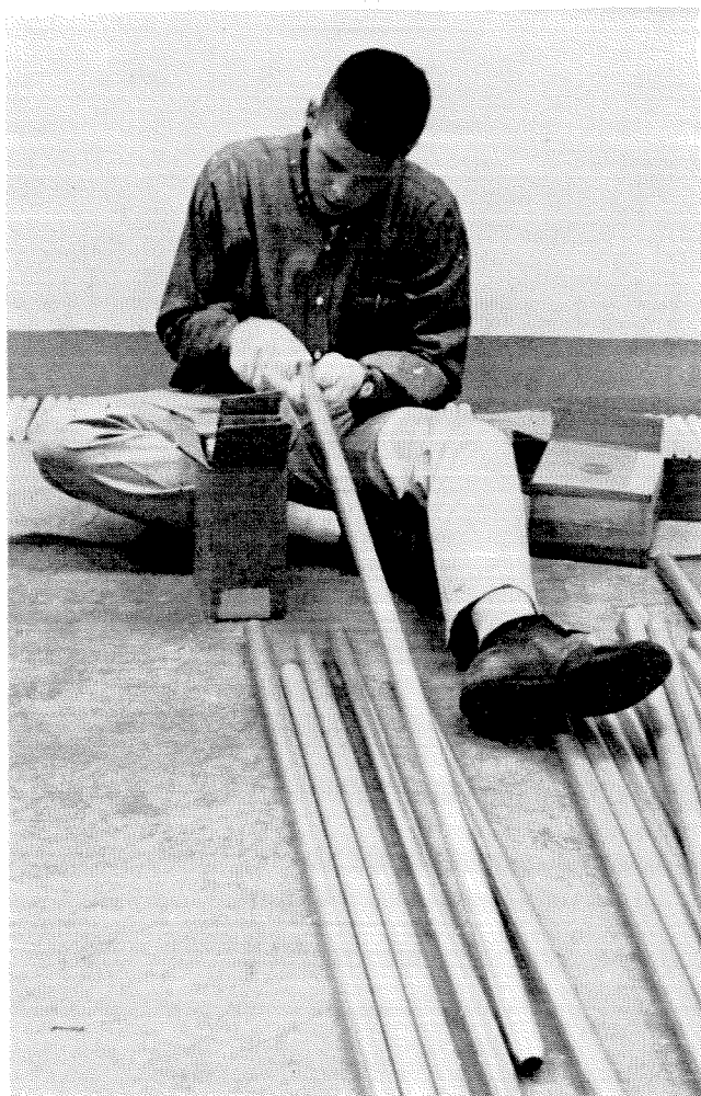
Five slugs of uranium are loaded into each of the 260 tubes that go into the atomic reactor. The uranium, valued at $100,000, is an AEC loan.
