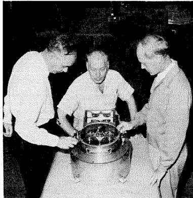
Fred Birri, superintendent; Frank Tennant, precision machinist; and Robert Harrington, engineer-designer, examine a new CES instrument. This is a dual viscometer, which measures the viscosity of liquids used in basic studies of hydrodynamics.
