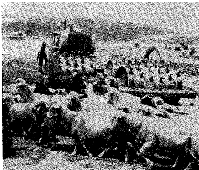
The sheep's foot roller — a widely-used compaction device — meets up with its natural inspiration.
