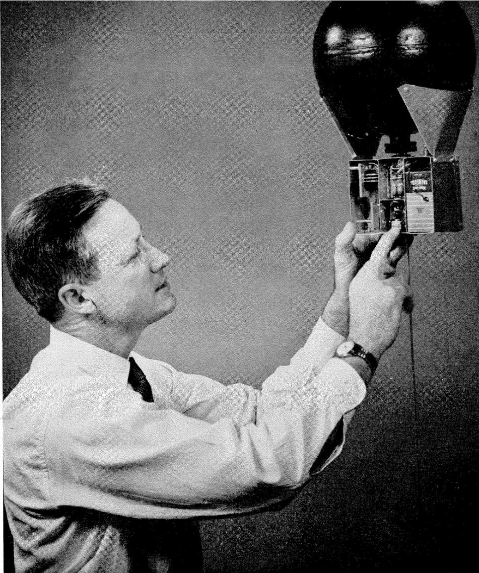
*Victor Neher, professor of physics, with the ionization chamber for measuring cosmic rays which is carried up to high altitudes by balloons. The chambers are used mainly in Polar regions, where cosmic rays are most intense.*
