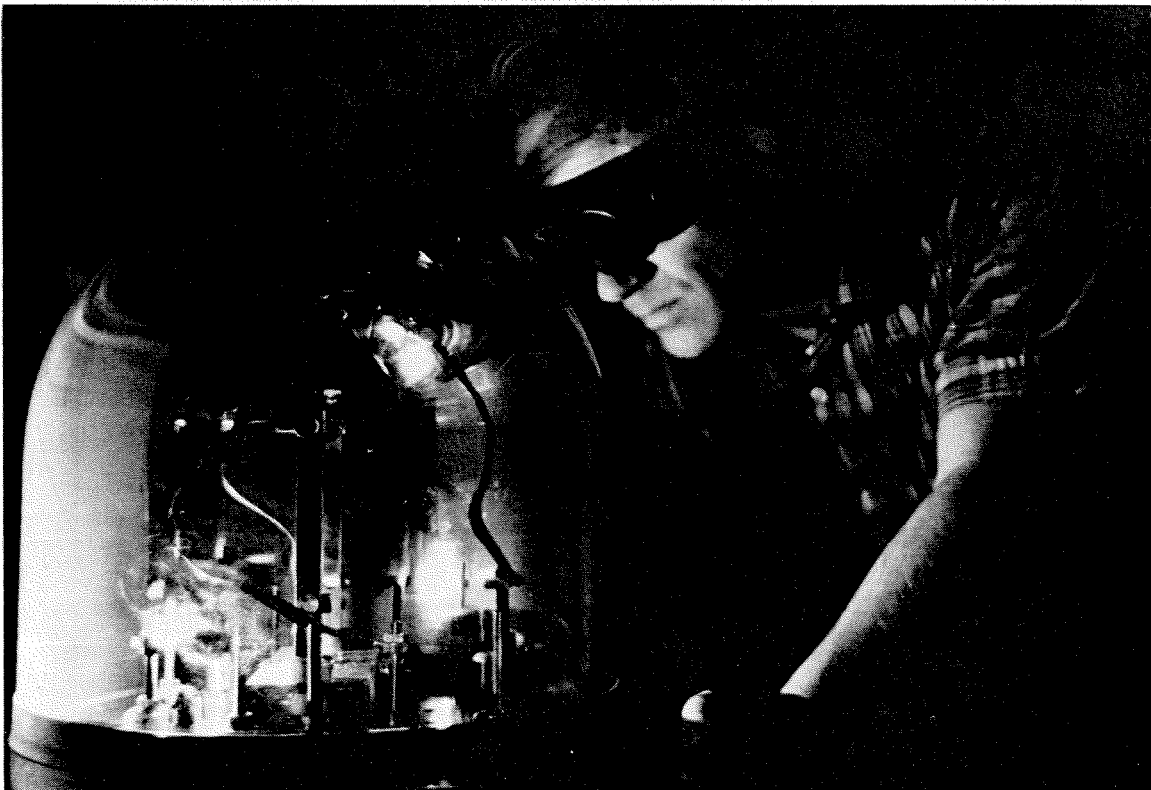
Before viruses or thin slices of tissue can be photographed with the electron microscope, a thin film of carbon must be deposited in this vacuum evaporator in order to support the specimen. Here, too, thin films of heavy metal elements are sometimes deposited on the specimens to enhance contrast in the negatives.
