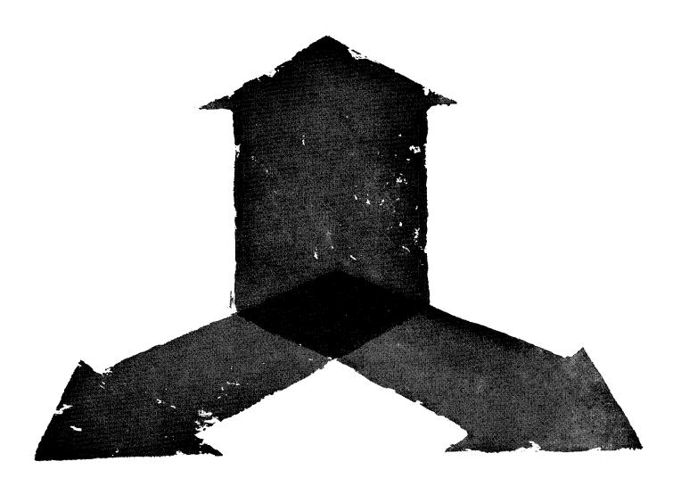
**Said Hans Oersted:** "When a conductor carries current through a magnetic field at right angles to it, the resultant reaction thrusts the conductor in a direction perpendicular to both the current and the magnetic field."
