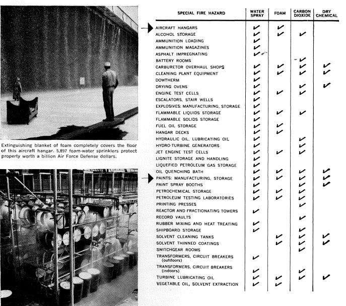
Water spray, applied to outside storage of paints and solvents, cools to inhibit internal pressure build-up and dilutes to prevent flammable vapor-air mixtures from developing. There's a Grinnell Fire Protection System to protect every type of property. Grinnell designed and installed systems are backed by over 90 years of fire protection experience. Grinnell Company, Providence 1, Rhode Island.
