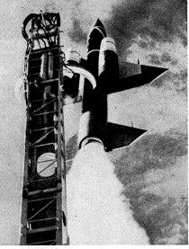
Supersonic Boeing BOMARC, longest-range air defense missile in U.S. Air Force arsenal, is now operational at Air Defense Command bases. New "B" model has range of more than 400 miles.
