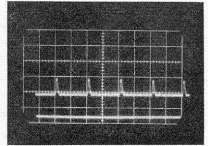
Right: Photocell record of the light emitted by the ruby when pulsing is controlled by a Kerr cell at 500,000 per second.
