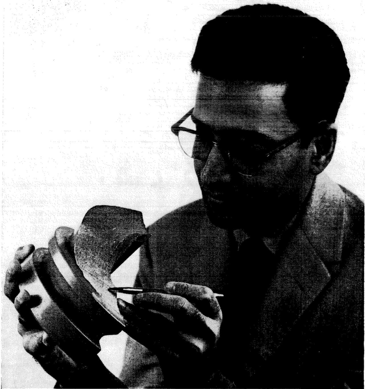
*Sitaram Valluri, senior research fellow in aeronautics, in a practical demonstration of his new theory, studies the aluminum alloy hub of a large propeller blade that failed because of metal fatigue. The blade ripped*
