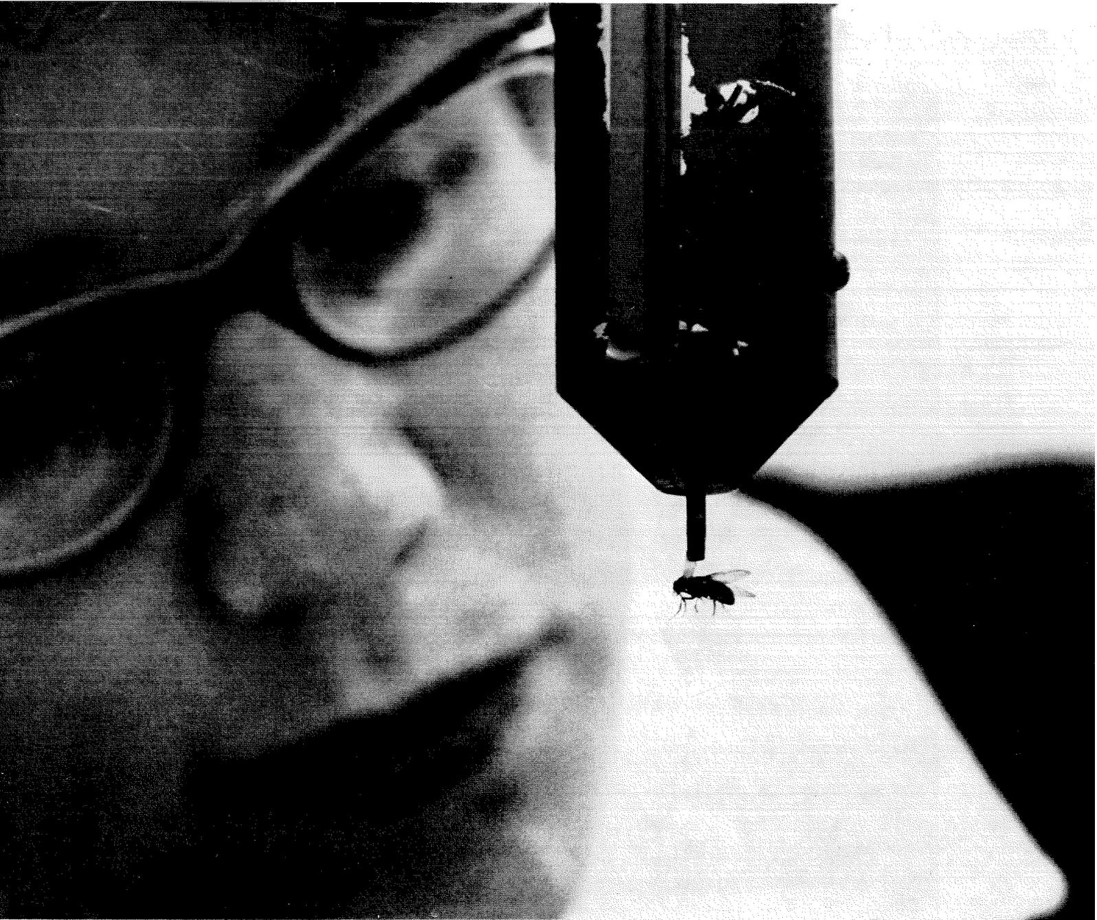
*Housefly, attached to torque meter which measures wingbeat response as the fly tries to follow a visual target*
