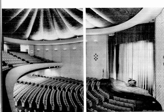
The interior of the auditorium is dramatically decorated in red, white, and gold. The ceiling, made of anodized aluminum discs attached to fiberglass tape, gives the effect of a filigreed gold curtain.
