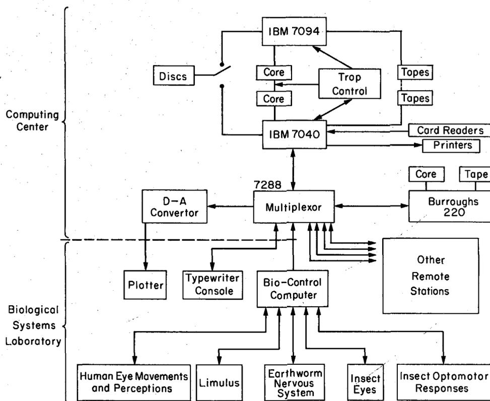
two computers is achieved by four interconnections; the computers are interconnected through 25 million words of tape memory, 18.5 million words of disc memory, 64,000 words of core memory, and an instantaneous trap control.
