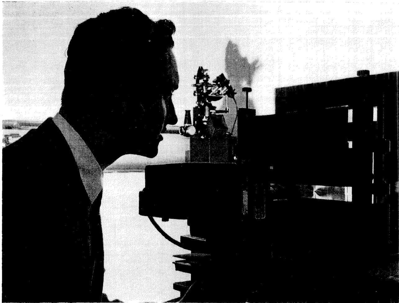
Wolfgang Knauss, research fellow in aeronautics, uses a sheet-straining device to measure the amount of energy that is dissipated when a fracture occurs in polymeric material.
