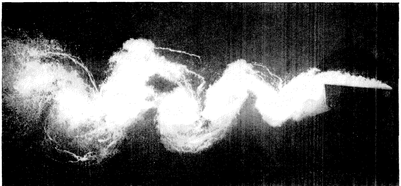
Cavitating wake behind a flat hydrofoil, just at the beginning of cavitation.
