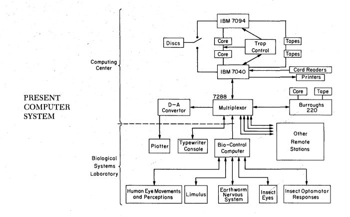
two computers is achieved by four interconnections; the computers are interconnected through 25 million words of tape memory, 18.5 million words of disc memory, 64,000 words of core memory, and an instantaneous trap control.
