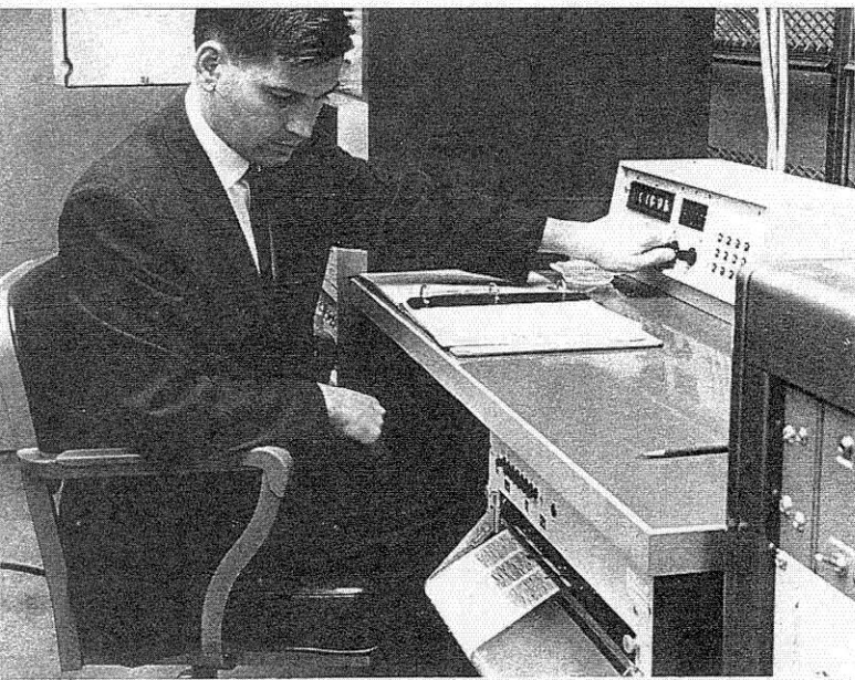
Stewart Smith, associate professor of geophysics, feeds data into a remote console connecting the computer and the Seismological Laboratory. The computer aids in determining the magnitude and location of earthquakes.
