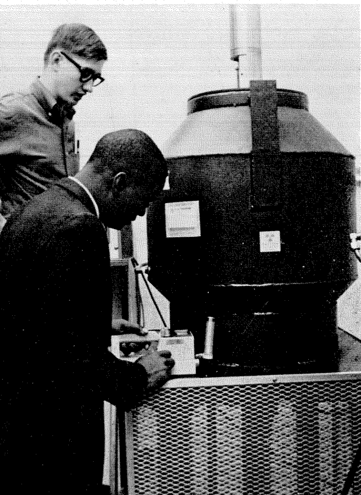
James King Jr., JPL research group supervisor, uses a Geiger counter to check the radiation level around a cobalt-60 gamma ray source. This equipment is used in experiments at JPL done by chemistry graduate student Thomas Penner (upper left).
