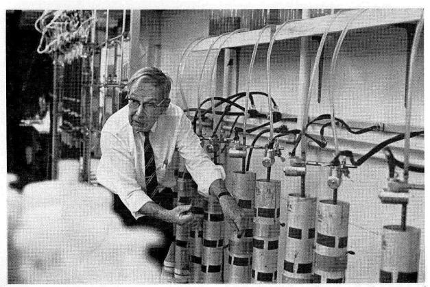
In water purification experiments conducted by James Harvey, sewage dumped into a complex system of aluminum tubes filters through sterilized sand and is then tested for fungi and bacteria.
