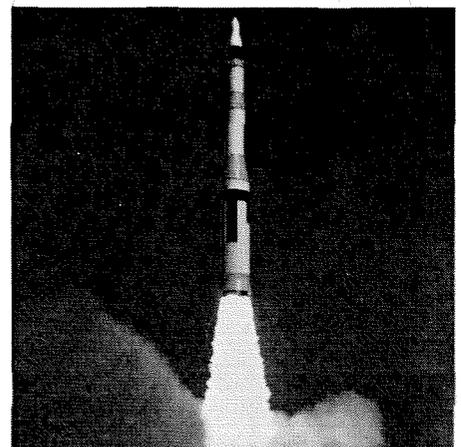
**USAF SRAM.** New U.S. Air Force short-range attack missile, now being designed and developed by Boeing, is a supersonic air-to-ground missile with nuclear capability. Boeing also will serve as system integration and test contractor.
