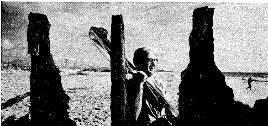
Vic holds a nickel-chrome plated automobile bumper which was tested in the corrosive seaside atmosphere.
