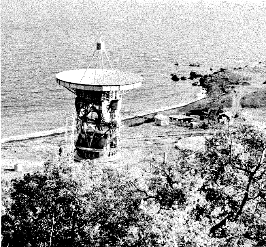
The 72-foot dish at the Crimean Astrophysical Observatory on the Black Sea—the eastern end of the 6,000-mile interferometer base line.
